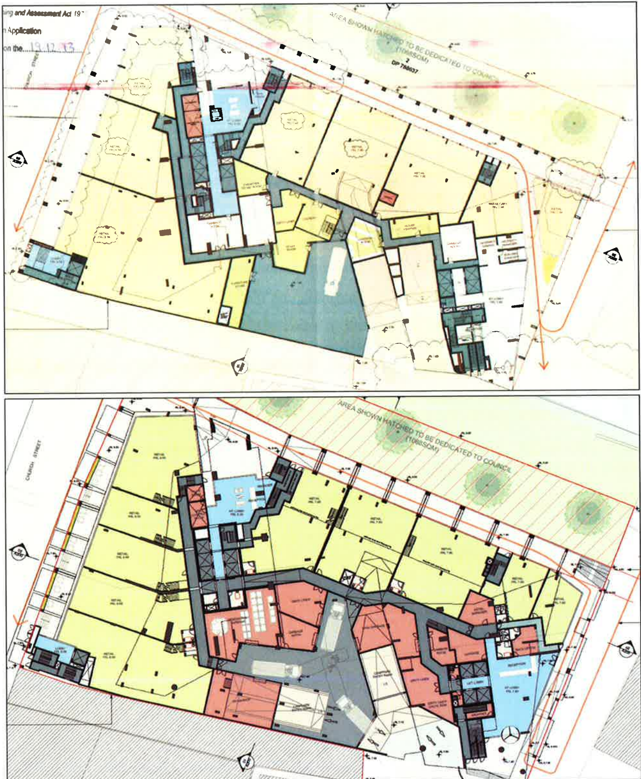
Figure 2: Approved (top) and proposed (bottom) ground floor retail, servicing and entrance lobby area layouts (Source: MP10_0171 MOD3 and proponent's application)
