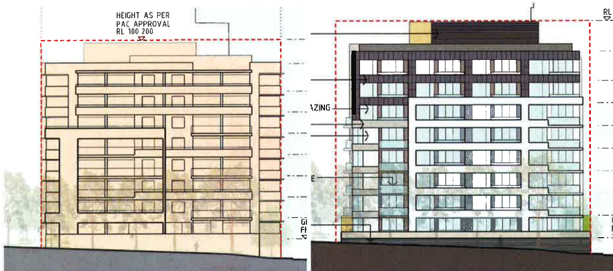
Figure 16: Northern elevation of Building Y / the Darwin Building – as approved (left) and proposed (right)
