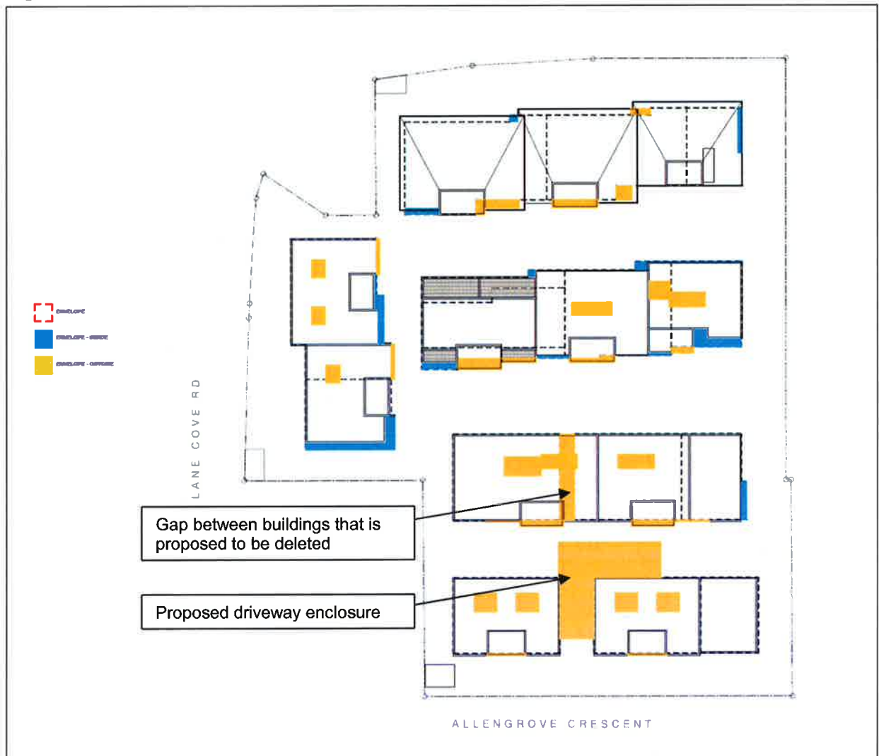
Figure 2 – Proposed changes to building envelopes – Roof level
