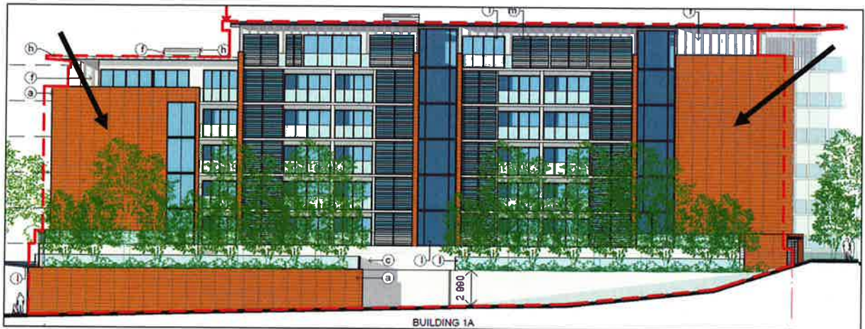
Figure 21: East elevation of northern site showing two large unbroken sections of wall which would benefit from improved articulation to reduce the appearance of visual bulk.
