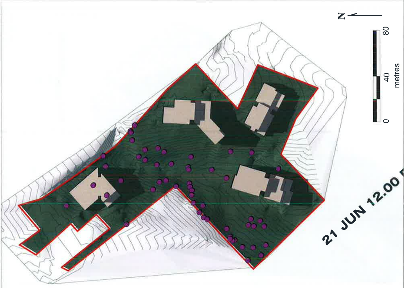
Figure 2d-8. Seasonal shadow diagram from natural topography (left) and from natural topography with proposed buildings (right)
