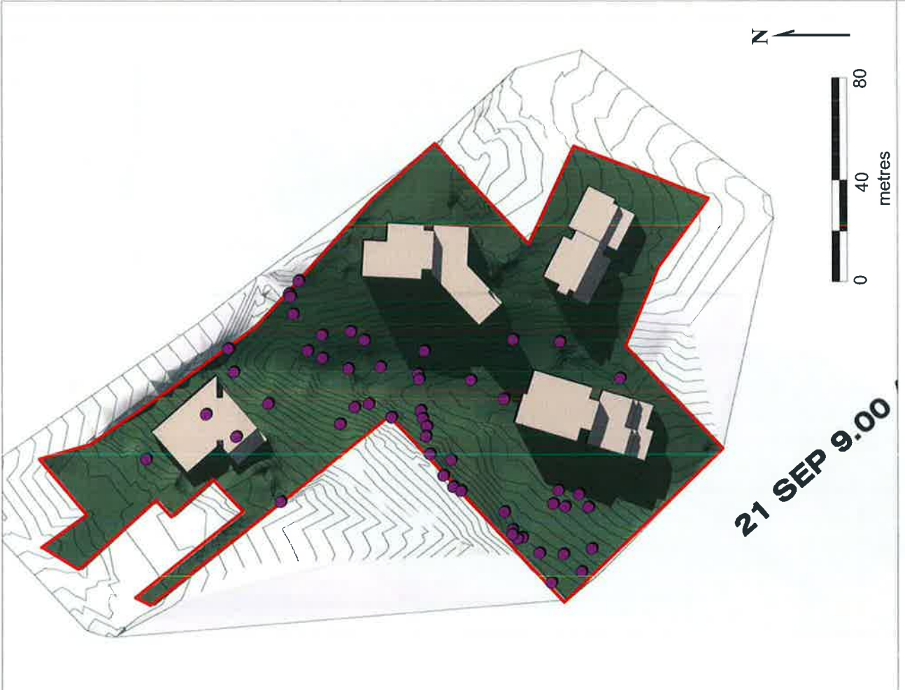
Figure 2d-10. Seasonal shadow diagram from natural topography (left) and from natural topography with proposed buildings (right)
