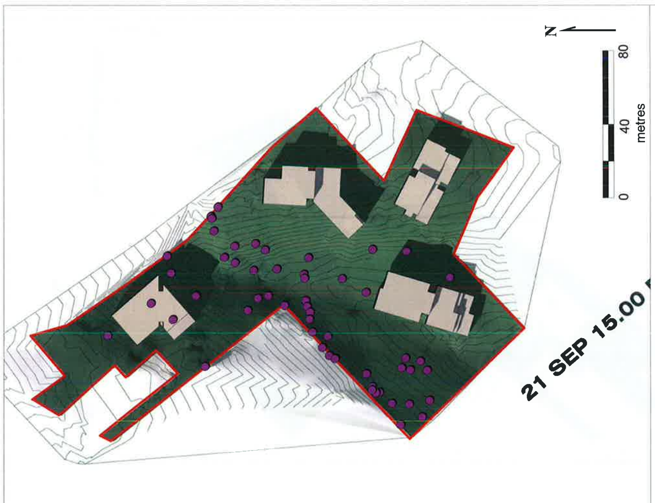
Figure 2d-12. Seasonal shadow diagram from natural topography (left) and from natural topography with proposed buildings (right)
