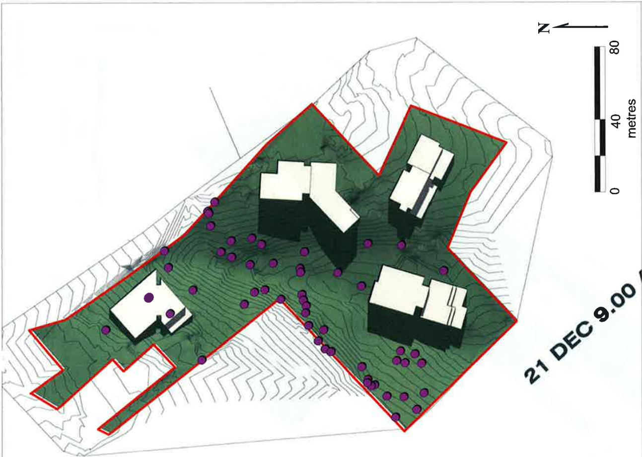
Figure 2d-1. Seasonal shadow diagram from natural topography (left) and from natural topography with proposed buildings (right)
