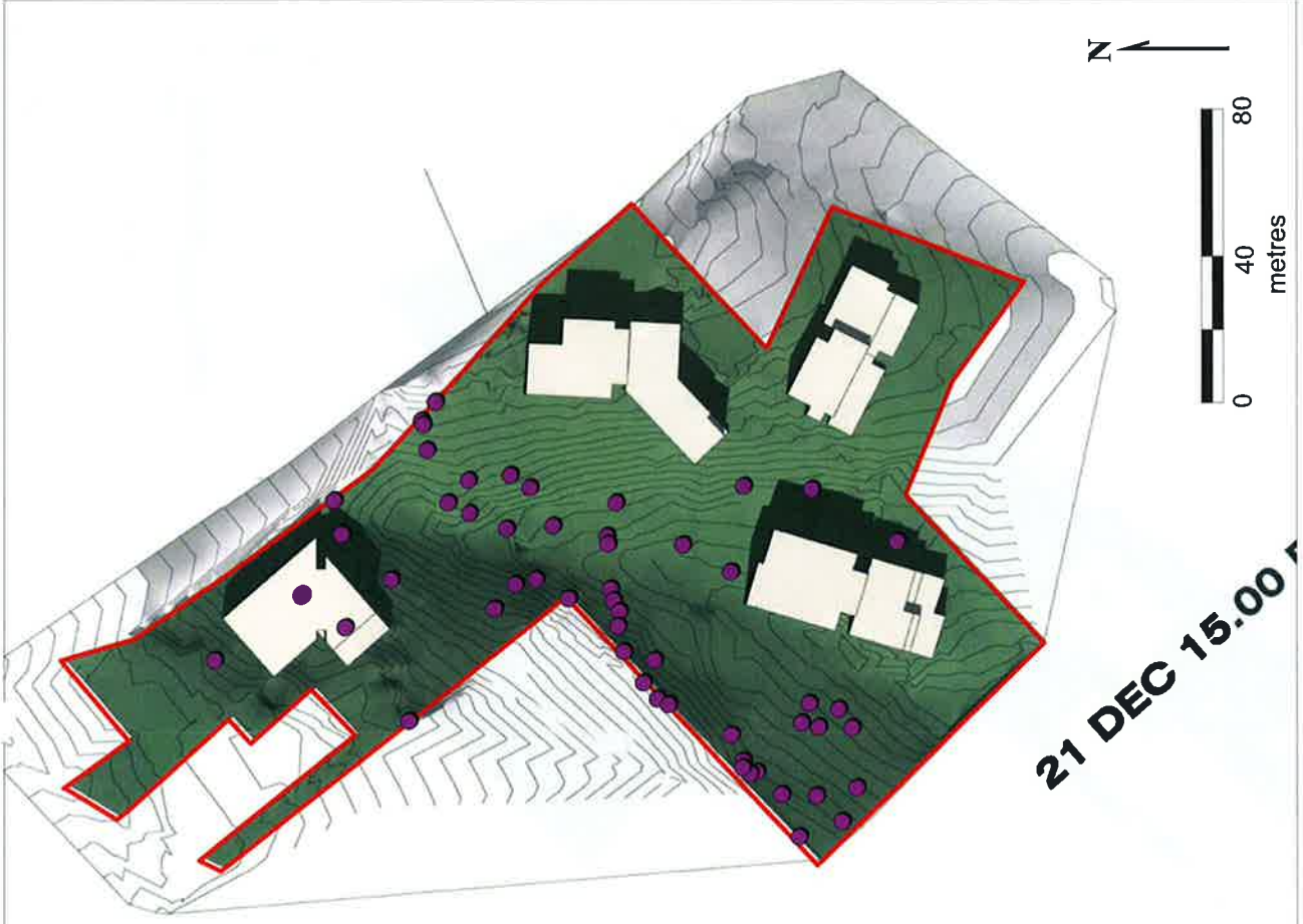
Figure 2d-3. Seasonal shadow diagram from natural topography (left) and from natural topography with proposed buildings (right)
