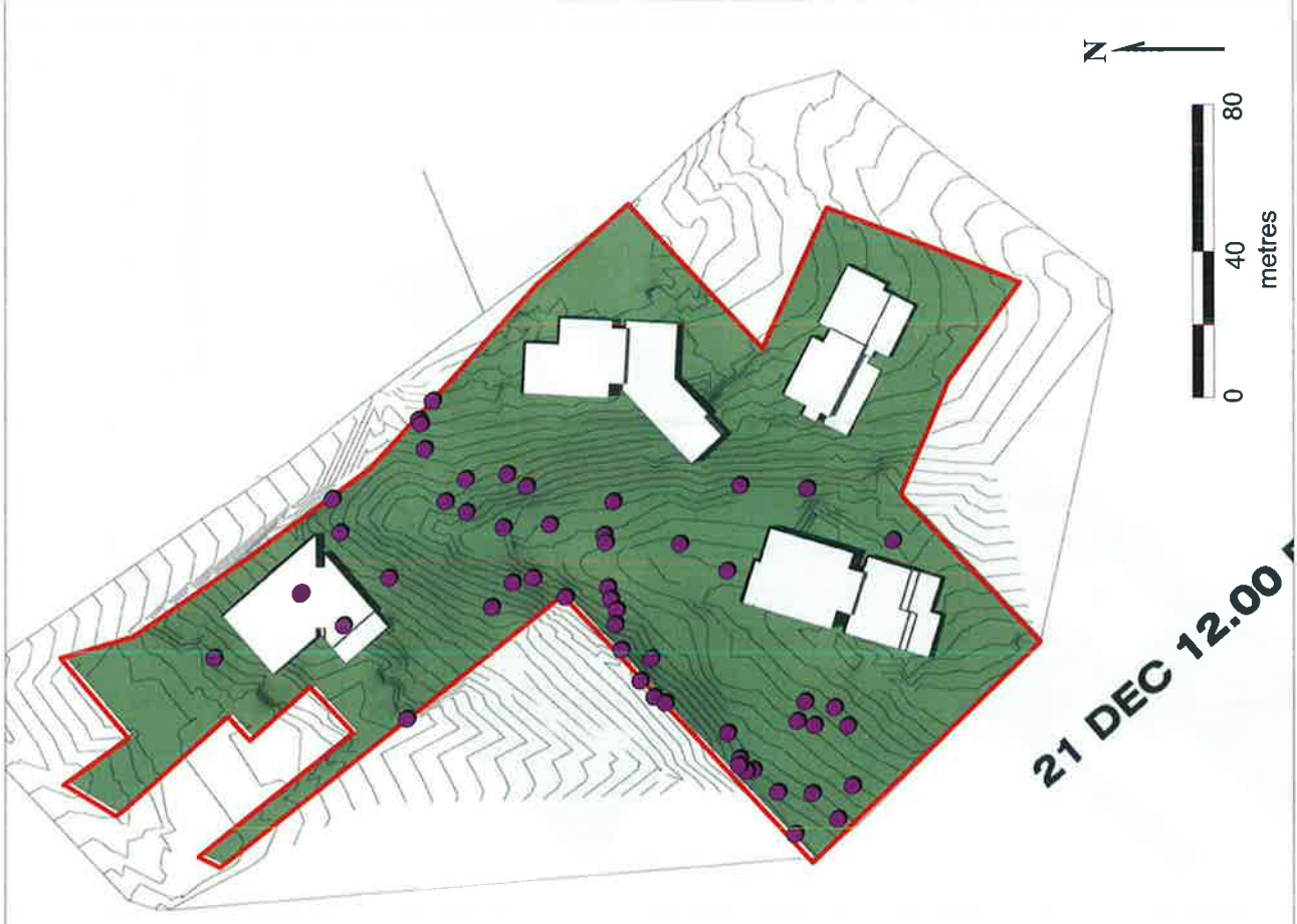
Figure 2d-2. Seasonal shadow diagram from natural topography (left) and from natural topography with proposed buildings (right)
