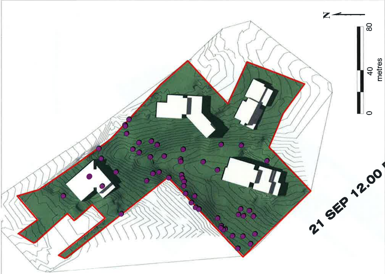
Figure 2d-11. Seasonal shadow diagram from natural topography (left) and from natural topography with proposed buildings (right)
