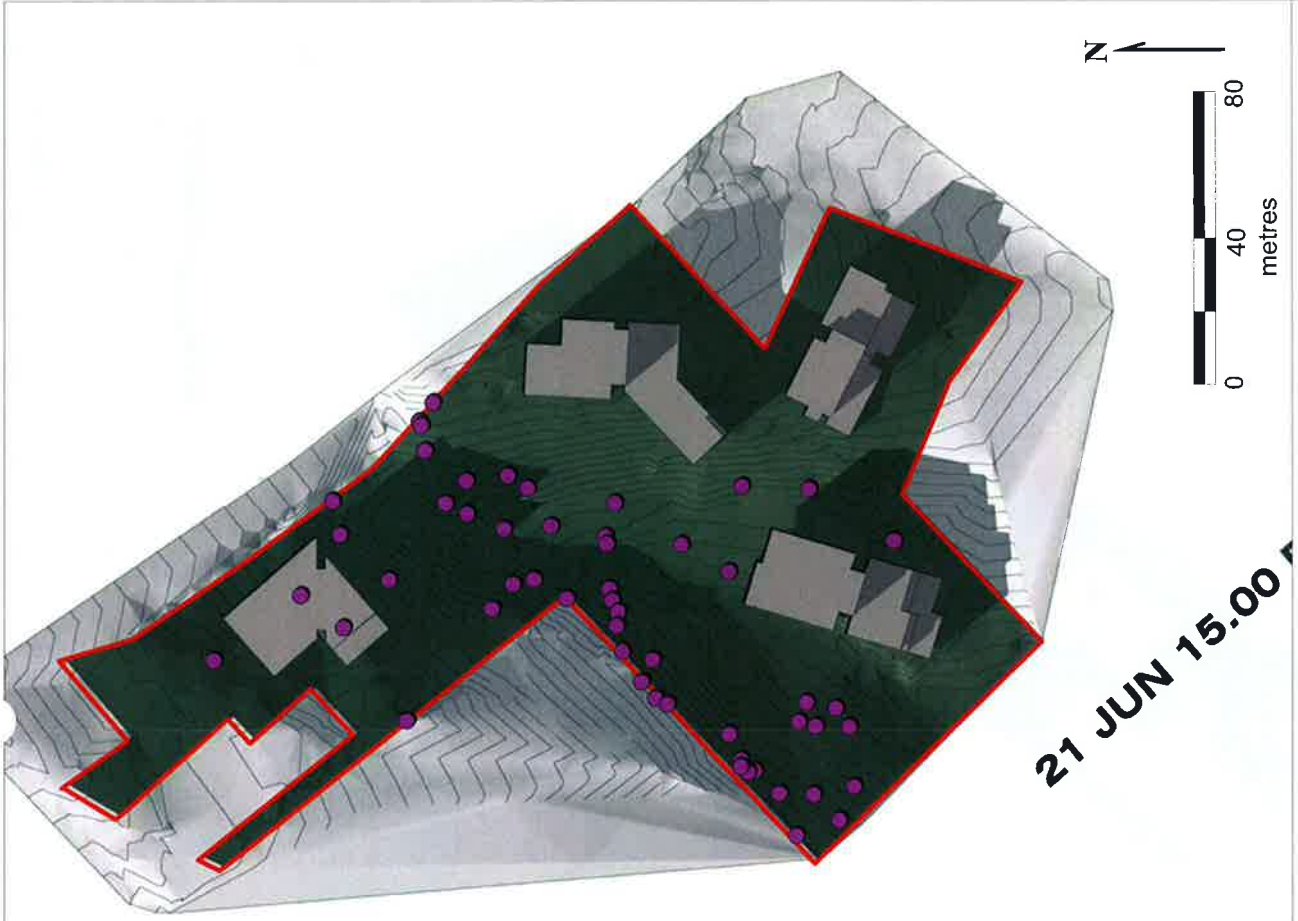
Figure 2d-9. Seasonal shadow diagram from natural topography (left) and from natural topography with proposed buildings (right)
