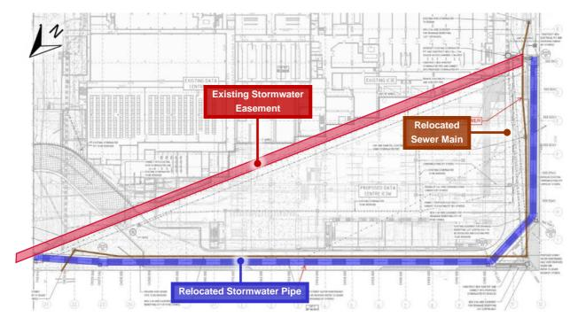
Figure 14 | Location of the relocated stormwater pipe and sewer main
