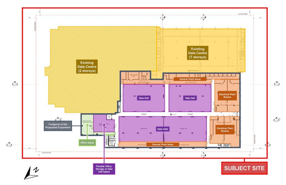
Figure 7 | Typical development layout (Levels 3-5)
