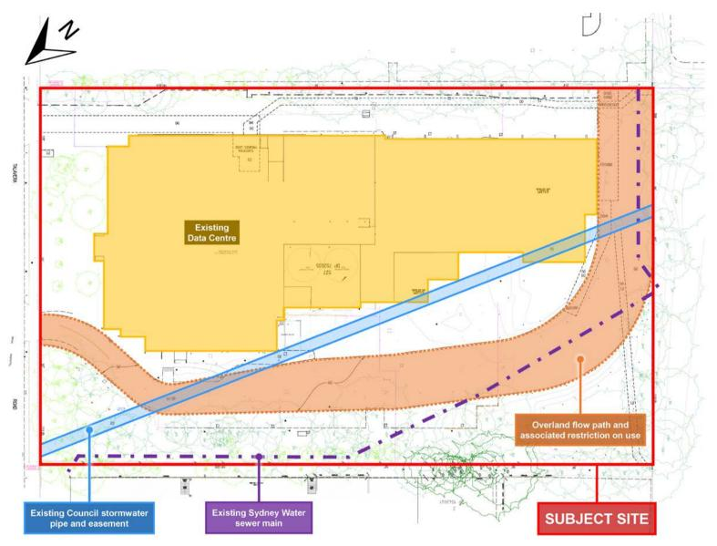
Figure 3 | Current survey plan, with key restrictions highlighted
